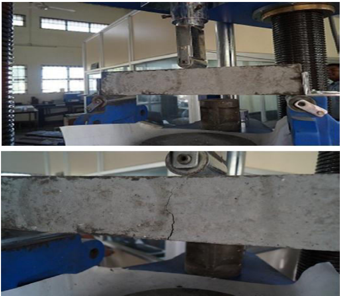
Figure 4.17: Flexural Strength tests of beam samples in UTM
