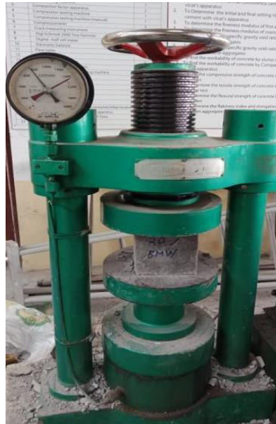
Figure 4.16: Compressive Strength test of cube sample
